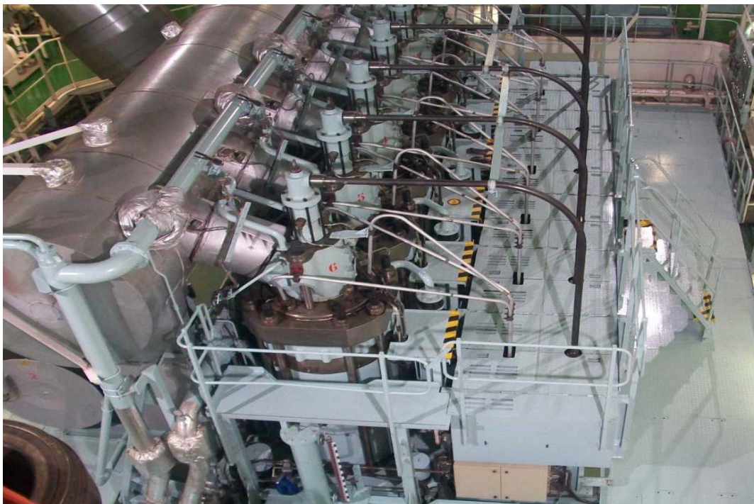
RT-Flex 68T-B, Minerva Nounou, (17.647 KW – 94 RPM)
